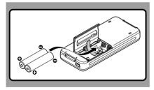
Insert the batteries in the direction inscribed on the inside of the recorder's battery compartment. In addition, when inserting the batteries, insert them so that the tape is under the batteries, as shown in the illustration. The batteries can then be removed easily by pulling up the tape. When pulling on the tape the batteries may suddenly pop out, so be sure to press down lightly on the batteries with your finger while pulling.
